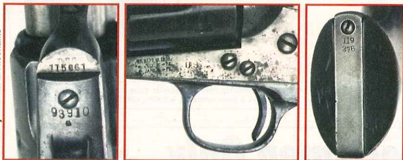
Trooper Bishop's revolver, as it is now, does not have matching numbers. It was returned to Colt in 1901 and was disassembled and refurbished. On reassembly, little attention was paid to matching the parts. Sub-Inspector David F. Clark's initials—"D.F.C."—are visible on the front of the frame (I).
